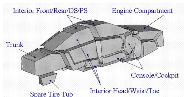
Figure 2: Typical cavities partitioning of an AutoSEA2 sedan car template
